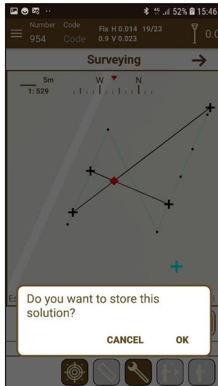
Figure 84. Intersection of two lines
