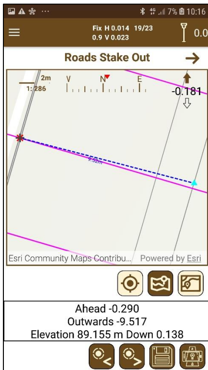
Figure 136. Road stake out (top view)
