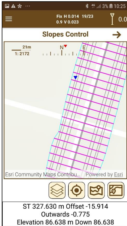
Figure 139. Slope control display (top view)
