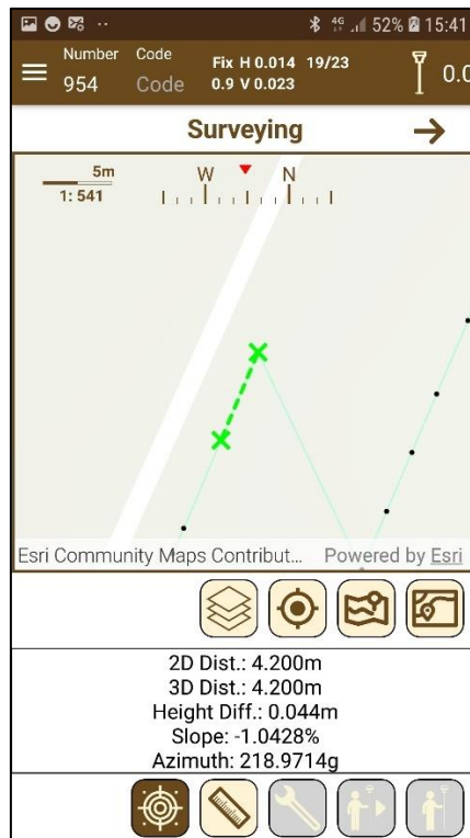
Figure 80. Measuring the distance between two points
