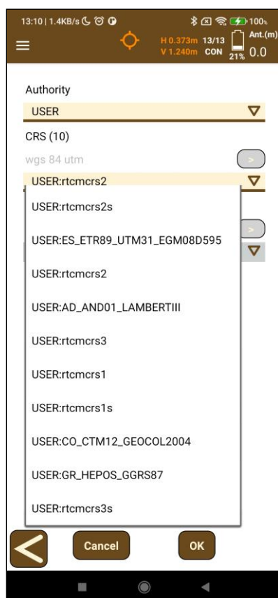
Figure 28. List of User CRS, including the created RTCM
